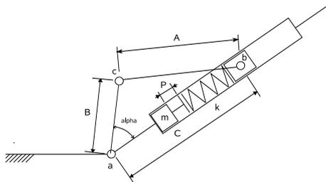
Figure 1: MACCEPA using rigid linkages.
