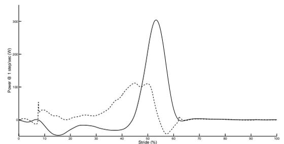
Figure 2: Ankle power during one gait cycle: Healthy ankle (solid line), motor (dashed line).
